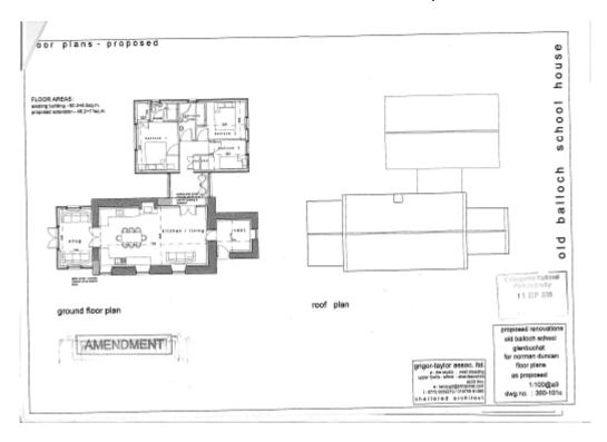
Figure 6 Proposed floor plans for the conversion and extension.
