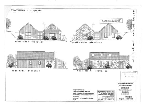
Figure 5 Elevations of the proposed conversion and extension.
